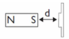
Care should be taken to make sure that the distance of magnet wheel to Hall Effect will be consistent over the long term. Systemic erosion of structures must be factored to prevent the wheel from eventually finding itself outside the maximum 18 mm distance gap from the Hall Effect sensor.
