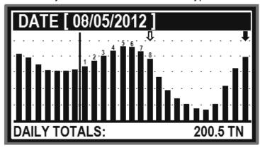
The user can view the daily totals by moving the arrow to the date of interest. The graph indicates that the daily total for 08/05/2012 was 200.5 TN. New data is always added on the right while older data is shifted to the left. A vertical line indicates the month separator. **Press CLEAR to exit the graphics plot function**
