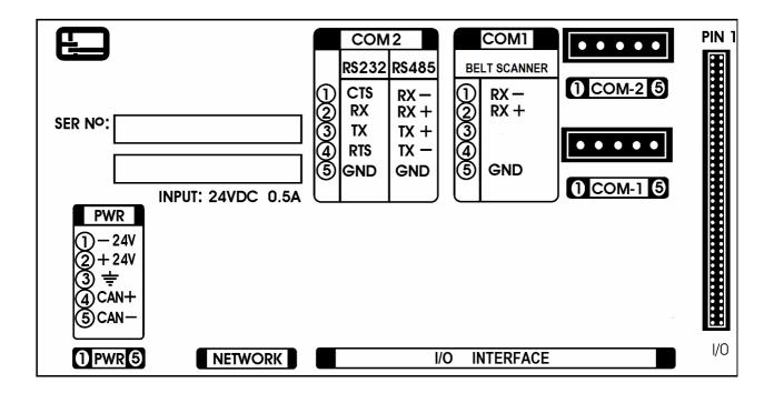
Power supply input. The indicator accepts a dc voltage between[16-48]Volts. If PoE is used, do not connect power 1 PWR 5 Nominal power input should be 24Vdc @ 200mA The controller supports three types of network **NETWORK** configurations. Ethernet, Wi-Fi or USB. The Ethernet option also supports PoE (power over Ethernet). 0 CH-1 6 Not used. 1 COM-1 5 Optical Belt Scanner This serial port can be configured as RS232 or RS422 and 1 COM-2 5
