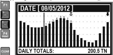
The user can view the daily totals by moving the arrow to the date of interest. The graph indicates that the daily total for 08/05/2012 was 200.5 TN. New data is always added on the right while older data is shifted to the left. A vertical line indicates the month separator. Press CLEAR to exit the graphics plot function
