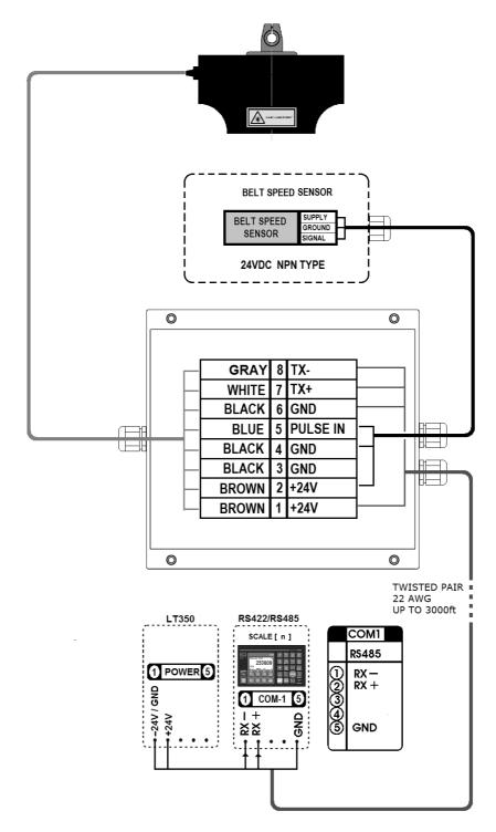
**NOTE:** When using static belt speed option, PULSE IN must be connected to ground in order for the totalizer to be active.
