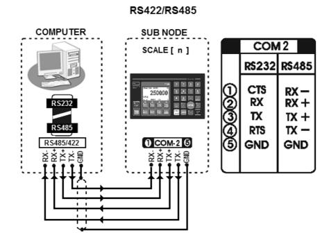
**NOTE:** A RS232 to RS422 converter is required for the computer
