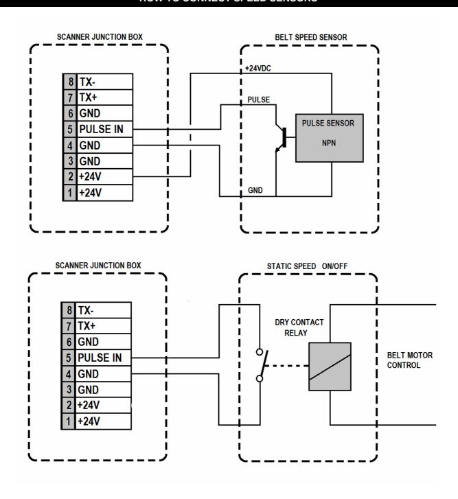
**NOTE:** When using static belt speed option, PULSE IN must be connected to ground in order for the totalizer to be active.
